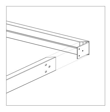
Layout one side (vertical) piece and the top and bottom (horizontal) pieces on smooth flat table.
