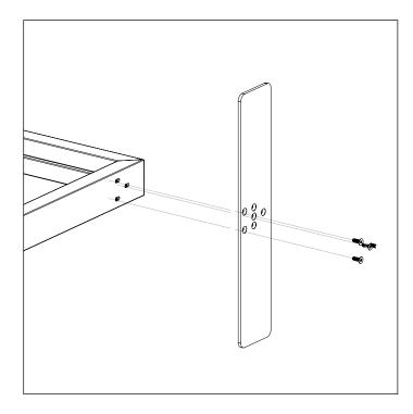
Use (3) button head screws to attach the top piece.
