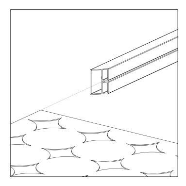
Slide panel into slot in frame.
