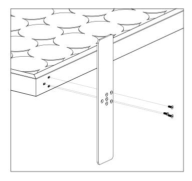
Use (3) button head screws to attach the top piece.
