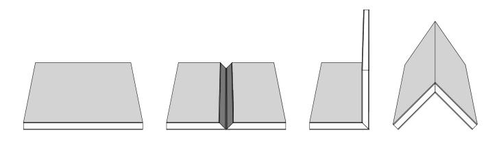
2. V-Groove and Miter Folding Example
